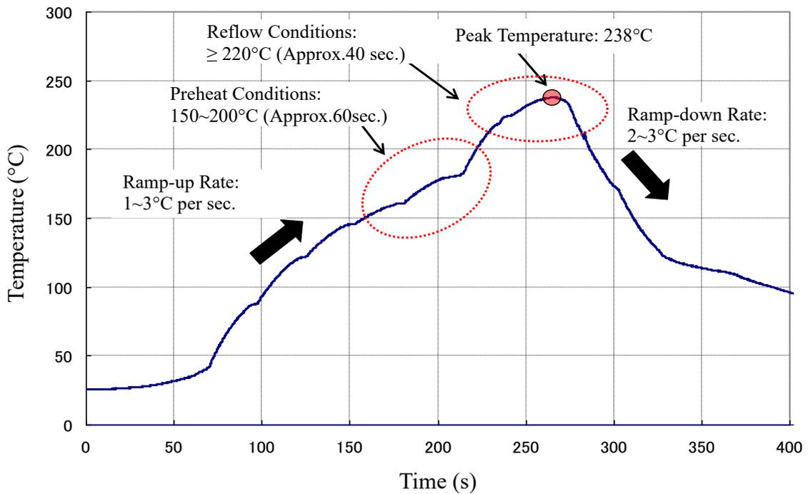
Figure 4. Actual temperature measured profile as target set-up for M705 paste
